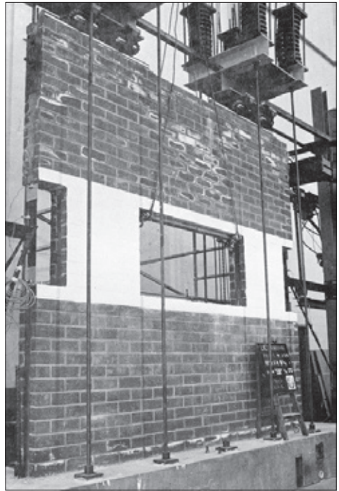
Masonry specimen ready for shake-table testing. Clough headed this mid-1970s project, along with graduate student Ron Mayes. Other graduate students working on the project were Polat Gulkan, Shy Chen, R. Hendrickson, George Manos, and Yutaro Omote.
