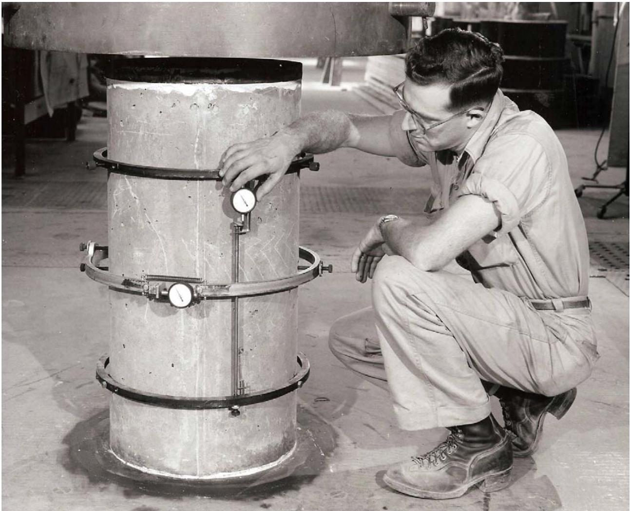
FIGURE 14 INSTRUMENTS TO DETERMINE LINEAR PROPERTIES OF CONCRETE
